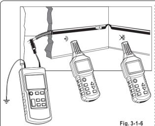
1.If there is current in the pipeline, cut off the power, and correctly earth it when the pipeline is not charged.
